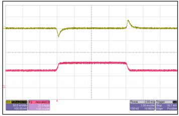
Figure 5: Output voltage response to step-change in load current (50%-100%-50% of lout(max);  $dI/dt = 0.1A/\mu s$ ). Load cap:  $15\mu F$  tantalum cap and  $1\mu F$  ceramic cap. Ch 1: Vout (50mV/div), Ch 2: Iout (20A/div).
