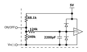
Figure B: Internal ON/OFF pin circuitry
