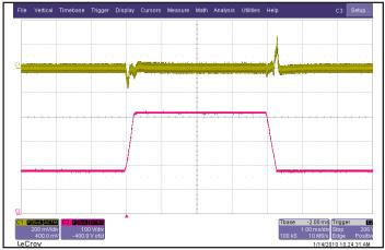
Figure 6: Output voltage response to step-change in input voltage (180V - 425V - 180V), at 50A load current. Load cap: 15µF tantalum capacitor and 1uF ceramic cap. Ch 1: Vout (200mV/div), Ch 2: Vin (100V/div).
