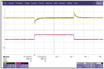
Figure 5: Output voltage response to step-change in load current (50%-75%-50% of Iout(max);  $dI/dt = 0.1A/\mu s$ ). Load cap:  $15\mu F$  tantalum cap and  $1\mu F$  ceramic cap. Ch 1: Vout (1V/div), Ch 2: Iout (2A/div).
