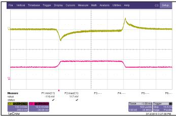
Figure 5: Output voltage response to step-change in load current (50%-75%-50% of lout(max);  $dI/dt = 0.1A/\mu s$ ). Load cap: 15 $\mu F$  tantalum cap and  $1\mu F$  ceramic cap. Ch 1: Vout (100mV/div), Ch 2: lout (20A/div).
