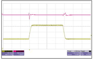
Figure 6: Output voltage response to step-change in input voltage (180V-425V-180V), at 60A load current. Load cap: 15µF tantalum capacitor and 1uF ceramic cap. Ch 1: Vout (500mV/div), Ch 2: Vin (100V/div).
