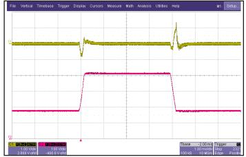
Figure 6: Output voltage response to step-change in input voltage (180V - 425V - 180V), at 6.25A load current. Load cap: 15µF tantalum capacitor and 1µF ceramic cap. Ch 1: Vout (1V/div), Ch 2: Vin (100V/div).
