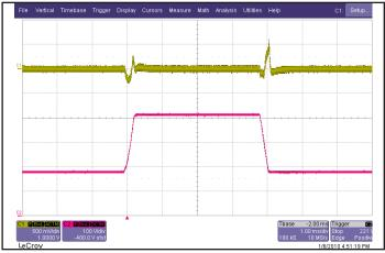
Figure 6: Output voltage response to step-change in input voltage (180V - 425V - 180V), at 12.5A load current. Load cap: 15µF tantalum capacitor and 1µF ceramic cap. Ch 1: Vout (500mV/div), Ch 2: Vin (100V/div).
