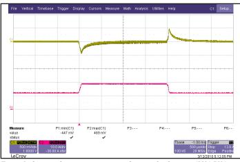
Figure 5: Output voltage response to step-change in load current (50%-75%-50% of lout(max);  $dI/dt = 0.1A/\mu s$ ). Load cap:  $15\mu F$  tantalum cap and  $1\mu F$  ceramic cap. Ch 1: Vout (1V/div), Ch 2: lout (5A/div).
