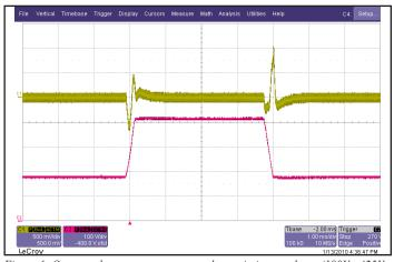
Figure 6: Output voltage response to step-change in input voltage (180V - 425V - 180V), at 10.7A load current. Load cap: 15µF tantalum capacitor and 1uF ceramic cap. Ch 1: Vout (500mV/div), Ch 2: Vin (100V/div).
