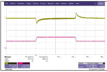
Figure 5: Output voltage response to step-change in load current (50%-75%-50% of Iout(max);  $dI/dt = 0.1A/\mu s$ ). Load cap:  $15\mu F$  tantalum cap and  $1\mu F$ ceramic cap. Ch 1: Vout (500mV/div), Ch 2: Iout (10A/div).
