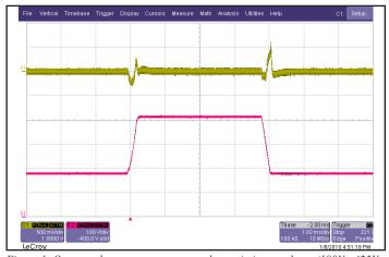
Figure 6: Output voltage response to step-change in input voltage (180V - 425V - 180V), at 20A load current. Load cap: 15µF tantalum capacitor and 1uF ceramic cap. Ch 1: Vout (500mV/div), Ch 2: Vin (100V/div).
