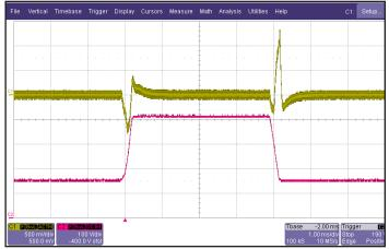
Figure 6: Output voltage response to step-change in input voltage (180V - 425V - 180V), at 6.25A load current. Load cap: 15µF tantalum capacitor and 1uF ceramic cap. Ch 1: Vout (1V/div), Ch 2: Vin (100V/div).
