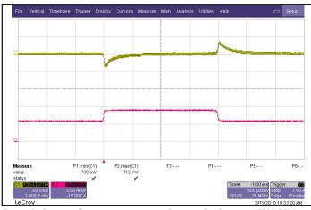
Figure 5: Output voltage response to step-change in load current (50%-75%-50% of Iout(max);  $dI/dt = 0.1A/\mu s$ ). Load cap:  $15\mu F$  tantalum cap and  $1\mu F$ ceramic cap. Ch 1: Vout (1V/div), Ch 2: Iout (5/div).
